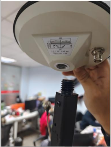
Install GNSS Antenna
