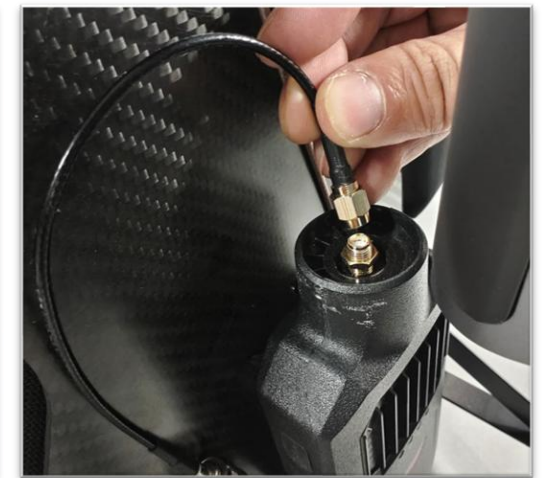
Install S-RTK100A and connect the feeder
