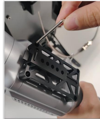
Install SLAM2000 bracket
