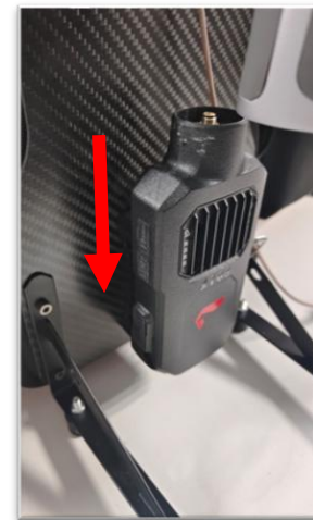
Install S-RTK100A and connect the feeder
